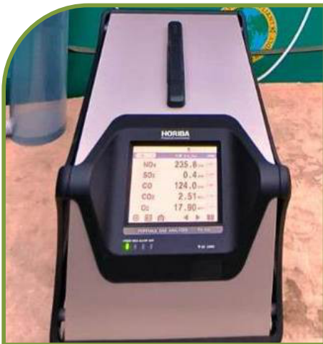
Flu-Gas Analyzer (M/S Horiba)
